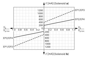
EP1/EP3 Technical data. EP2/EP4 Proportional solenoid Voltage 12 V (±20%) 24 V (±20%) Current limit 1.54 A 0.77 A Nominal resistance (at 20 °C) 5.5 Ω 22.7 Ω Dither 100 Hz 100 Hz frequency minimum oscillation range<sup>1)</sup> 240 mA 120 mA 100% 100% Duty cycle Type of protection: see connector version page 27
