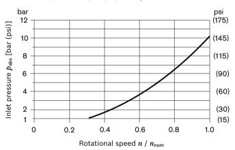
This diagram is only valid for the optimum viscosity range of  $v_{opt}$  = 36 to 16 mm<sup>2</sup>/s (170 to 73 SUS).
